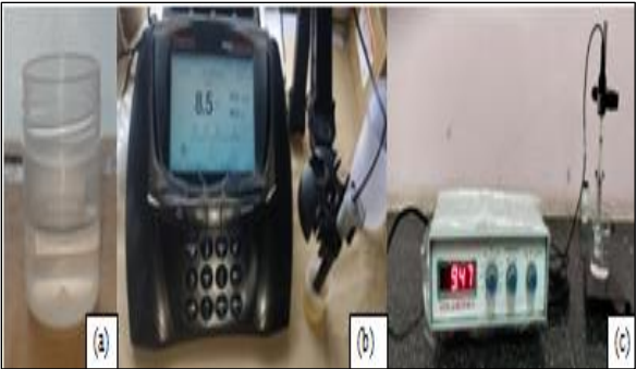
Figure 1: (a) Collection of ground water sample from Wadloor village of Raichur, (b) Ion selective electrode used for the estimation of fluoride level and (c) Estimation of pH of water sample.
