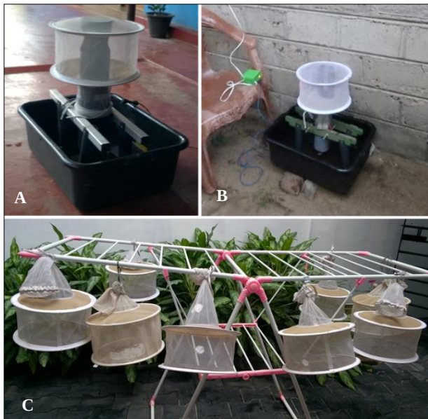
Figure 1 (A-C): Trapping and collection of mosquitoes by CDC gravid trap.
