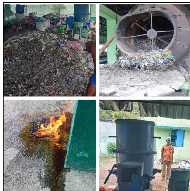
Figure 2: Conversion of plastic wastes to gasoline by a low-pressure pyrolysis plant in Chennai.
