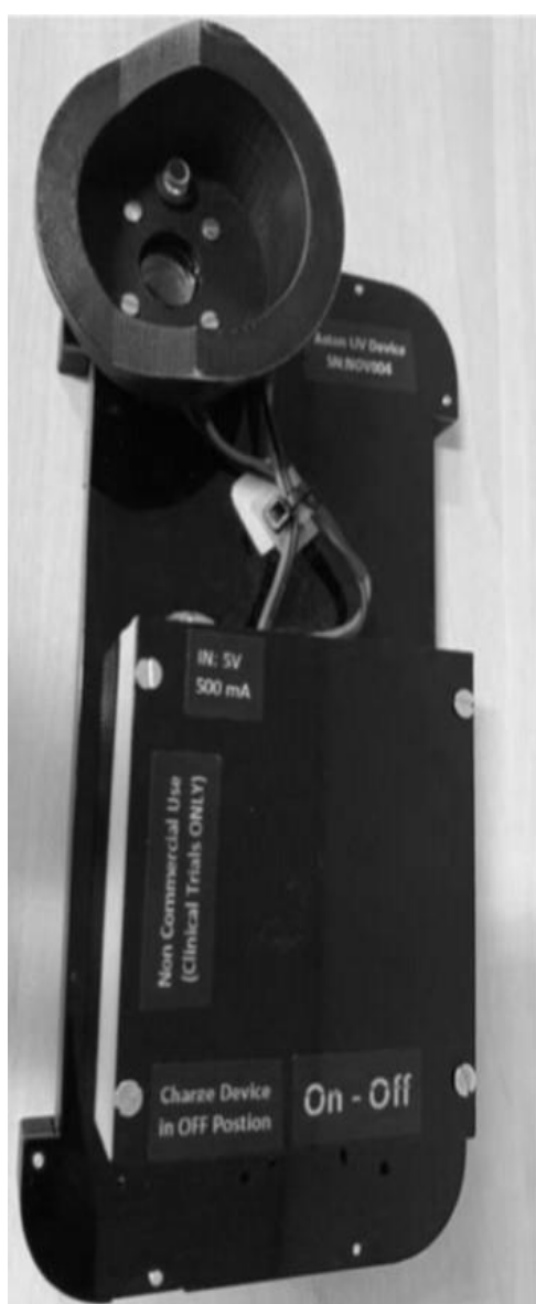
Figure 1: Novel iPhone fitted conjunctival ultraviolet autofluorescence photography system used to measure the conjunctival damage.
